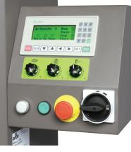
The control panel features a user-friendly display, knobs for turntable speed carriage speed and film tension, power light, start button, E-stop button and power disconnect.
