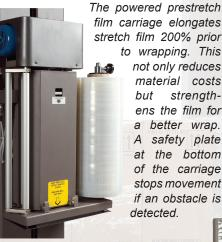
film carriage elongates stretch film 200% prior to wrapping. This not only reduces material costs but strengthens the film for a better wrap. A safety plate at the bottom of the carriage stops movement if an obstacle is detected.
