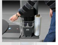
Loading stretch film is fast and easy. Just open the hinged door, pull the film tail through, and close the door. Power is automatically disconnected when the door is opened.
