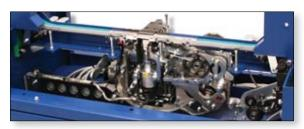
The new Standard-6 Sealer is fully accessible for faster cleaning with quickrelease tabletop
